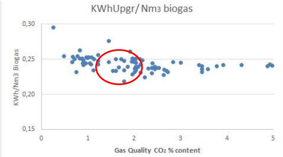
**Figure 5 Energy consumption versus CO<sub>2</sub> content in product gas**
