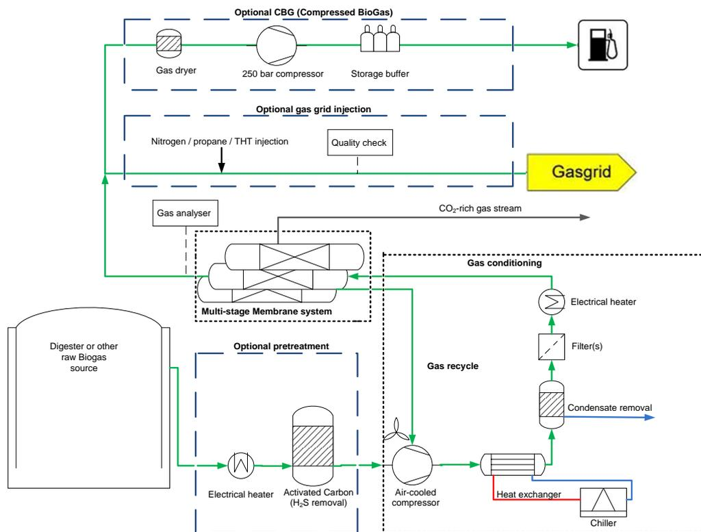
**Figure 2 Configuration of a typical DMT Carborex® MS system**
